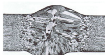
Grain growth after high heat input for in ferritic stainless steel welding
